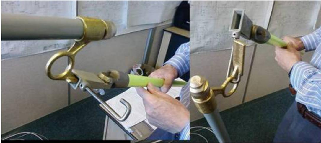
*Figure 3. The insertion tool to replace fuses / drop out surge arresters*
