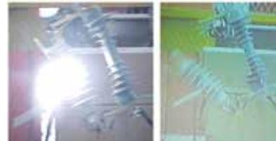
Figure 15: The operation of the surge arrester once it becomes faulty.
